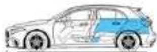
Open luggage compartment behind driver's seat, rear seat backrest folded, loaded to upper edge of driver's backrest, volume 825 litres (V 211-1)
