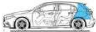
Open luggage compartment behind rear seat, loaded to roof, volume 435 litres (V 214-2)
