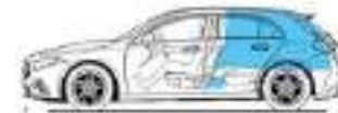
Open luggage compartment behind driver's seat, rear seat backrest folded, loaded to roof, volume 1,195 litres (V 214-1)
