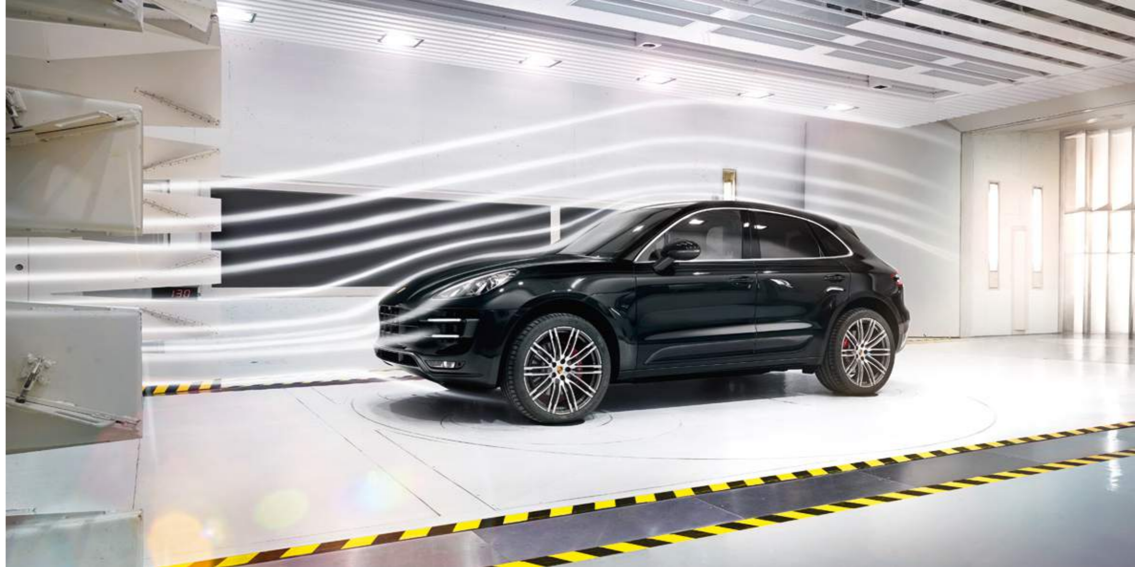
Wind tunnel in the Porsche Development Centre, Weissach
