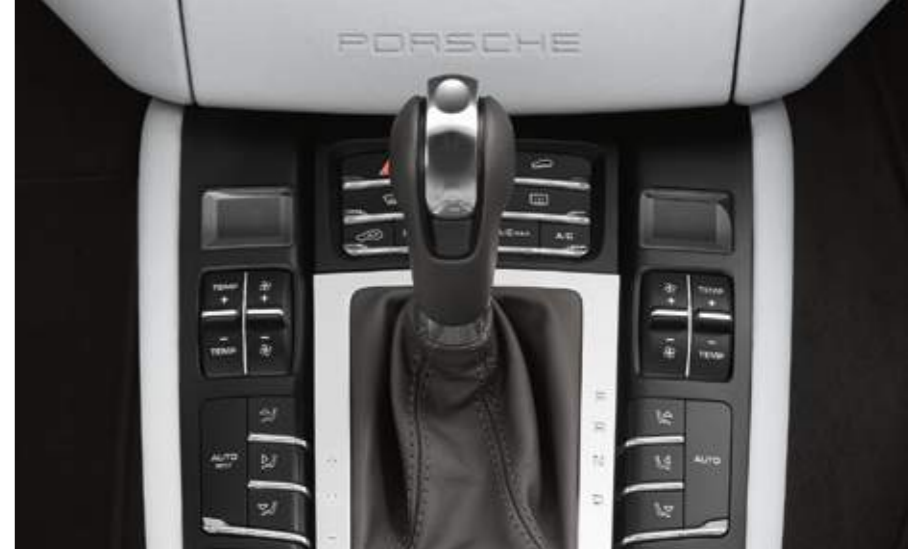
Climate control buttons in front for two- and three-zone automatic climate control
