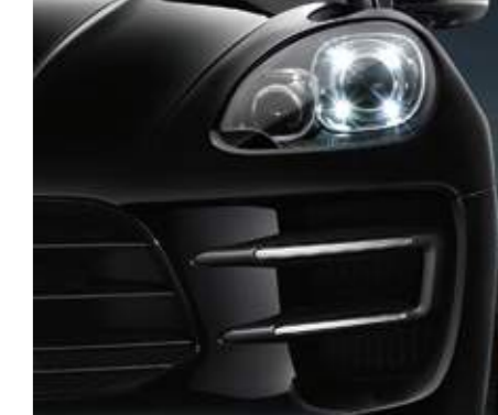
Daytime running lights with Bi-Xenon headlights
