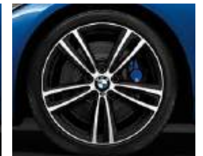
21C 19" M light alloy Double-spoke style 442 M, Bicolour Orbit Grey with mixed run-flat tyres, 8J x 19, 225/40 R19 front and 8.5J x 19, 255/35 R19 rear.
