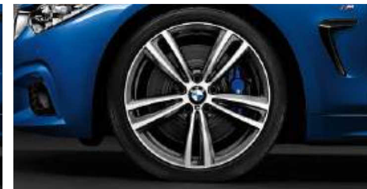
□ 23N 18" light alloy V-spoke style 398, Orbit Grey with performance tyres, 8J x 18, 225/45 R18 tyres front and 8.5J x 18, 255/40 R18 tyres rear.
