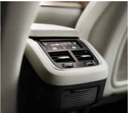
The four-zone climate system can be controlled from the center display touchscreen, or a graceful touch control panel at the end of the tunnel console.
