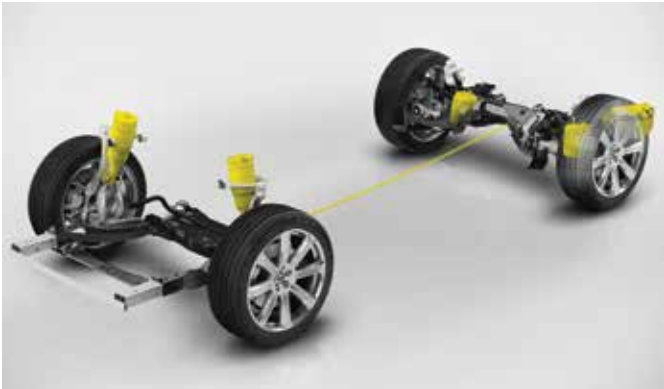
Choose the Off Road mode and the air suspension will raise the car by 1.6 ". Hill Descent Control is activated at the same time: the car brakes for you on steep gradients – all you need to do is steer. The Off Road mode gets your XC90 to navigate challenging terrain – all you need to do is turn the elegant drive mode selector to the desired position.
