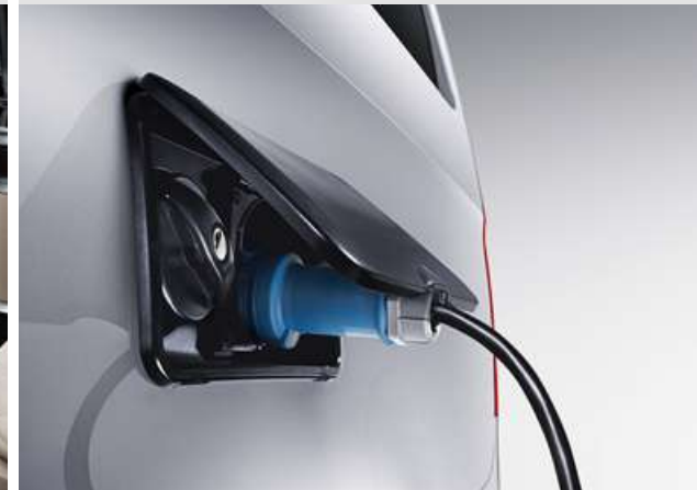
External connections for power and fresh water
