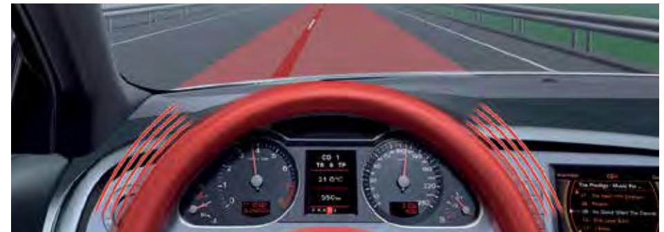
Audi active lane assist – steering wheel vibration
