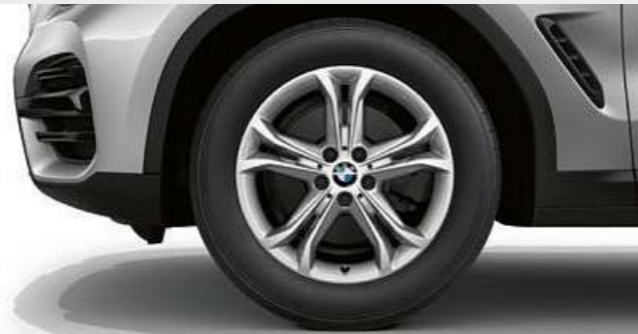
□ 18" light alloy Double-spoke style 688 wheels, wheel size 7J x 18 with 225/60 R18 tyres. (Standard for BMW X3 xDrive30d.)
