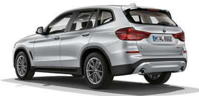
□ 18" light alloy Double-spoke style 688 wheels, wheel size 7J x 18 with 225/60 R18 tyres. (Standard for BMW X3 xDrive30d.)
